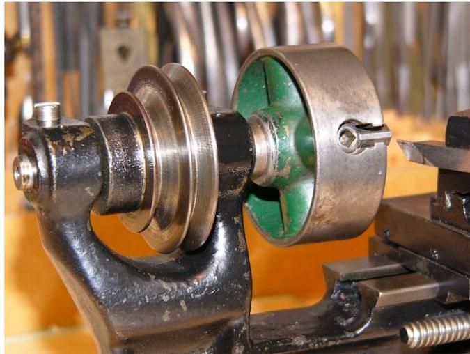
**Super Adept headstock. Short, solid spindle running in 3/8" iron housings without bushings. Note the light 4-jaw chuck. Collection A. Webster.**
