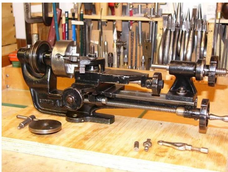
**Super Adept after restoration, sitting on a Peter Denny style 'kitchen table workbench' with Austerity period hand tools. Note (1) the splendid waisted handle on the lead screw hand wheel, (2) the long, blank taper in the tailstock's socket; the tailstock has a very short bearing surface for the barrel to slide in. Collection A. Webster.**
