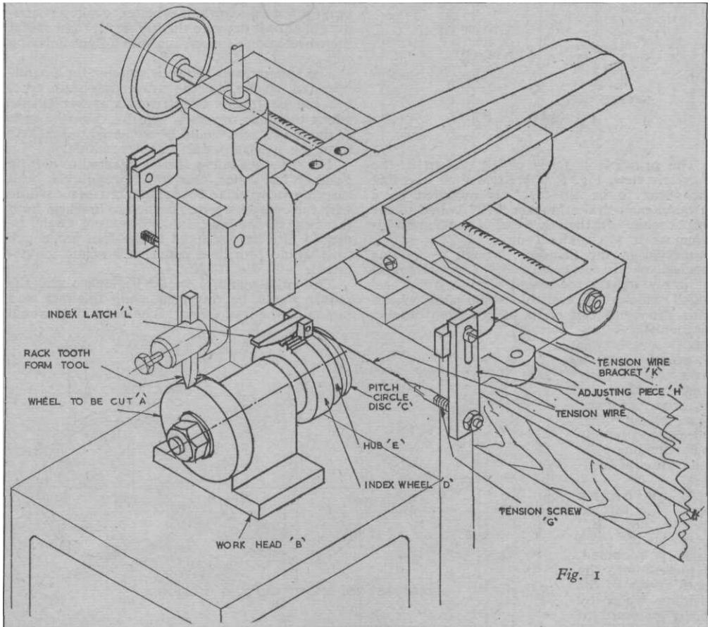
The idea is to use a shaping machine (in the writer's case, a very old hand-operated machine) and to fit to it a mechanism on the lines of that used in some types of gear-grinding machines, such as the "Maag" or older "Lees-Bradners" to give a rolling motion to the gear blank while being cut. This method, being a true generating method—right back to first principles—results in a correctly formed involute tooth.
