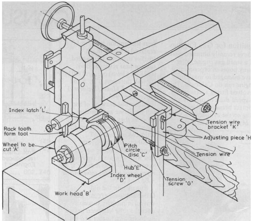
This is the drawing which was published as Fig. 1 of the original article by *Base Circle*, see text for an explanation.
