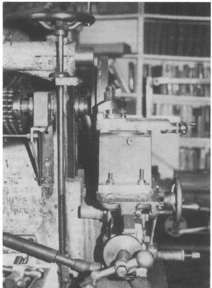
Having decided upon a method, the problem of producing the 96T blank had to be solved. This blank is 9.8 in. dia. and I proposed to machine it from a manhole cover casting. This, however was significantly larger than the 10 in. that my Myford Super 7 lathe will swing in the gap.
