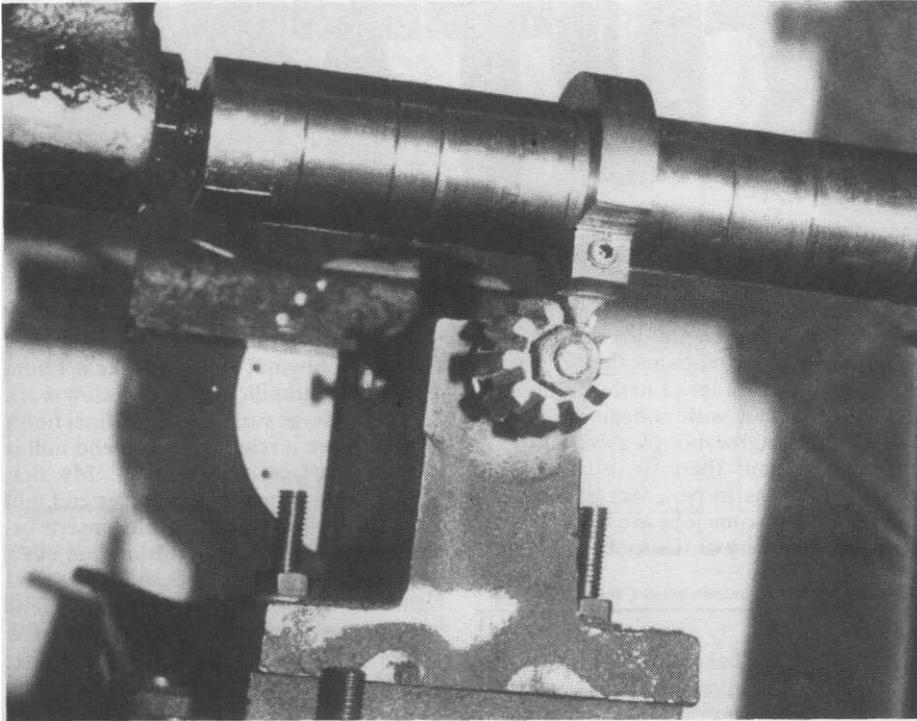
Above: Fig. 9 shows offset cutting. The cutter holder is offset by removing the washer, pinion rotated and indexed to the top hole in the angle.
