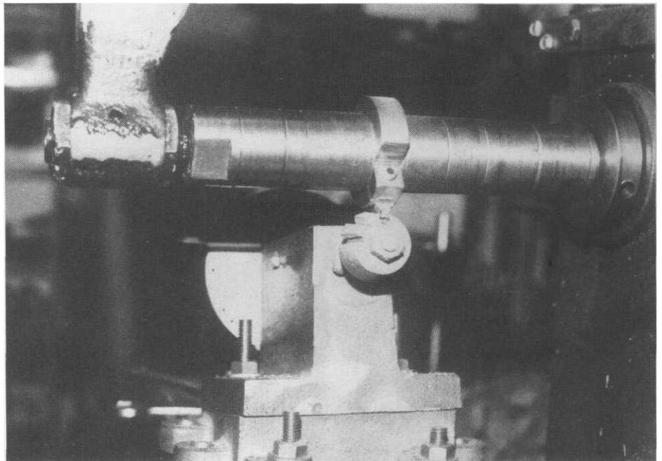
Above: Fig. 8 shows the set-up for pinions, tapered packing plate and blank holder.
